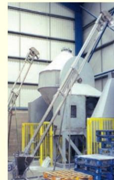
Portable conveyor feeding cone blender.
