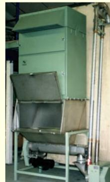
Vertical conveyor with bag dump station, screw feeder, and integral dust collection system.
