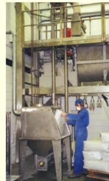
Manual bag dumping into vertical conveyor to feed mixer.
