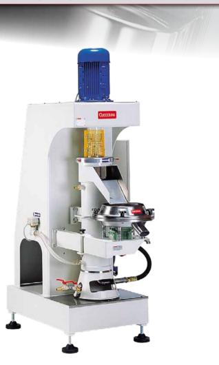
Refining mill with continuous operation and wet milling for printing pastes, colorants and ceramic glazes. The machine may have various levels of automation and control of the particle size. The use of micro milling balls in sintered alumina guarantees zero residue at
