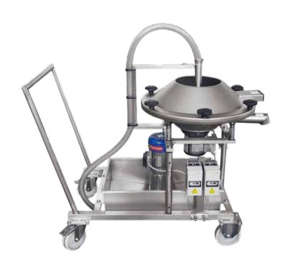
Wheel-mounted unit for sorting and screening glaze, engobe products and printing pastes on glazing lines. The tank with re-launch pump is used to screen the product returned from the belt scraper and from the "overflow" before putting it back in the service tank of the application unit.
