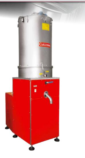
Double action refining mill (dispersion + milling) with discontinuous operation and wet milling for printing pastes, colorants and ceramic glaze. The belt transmission between motor and milling components, plus the inverter power supply, mean that large quantities of product can be dispersed and refined.
