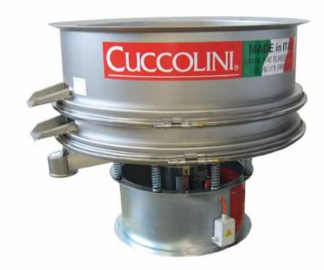
Circular sieve for slurry and dirty water in general. Part of the production range for over 25 years, it has been constantly up-dated through to reaching its present high level of reliability and performance. Vibrations keep the mesh constantly free from residues and enable the machine to work 24/7, with brief operator interventions to clean the meshes on a periodic basis.
