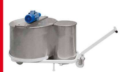
Glaze mixer suitable for feeding application units of glazing lines (i.e.: bells/discs etc). Thanks to the constant re-circulation of the product, you can obtain a perfect mix without any sediments. Its peculiar "8" shape enables the installation of the CPSV vertical pump.
