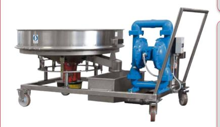
Wheel-mounted mobile unit for screening, transferring and removing iron from glaze.
