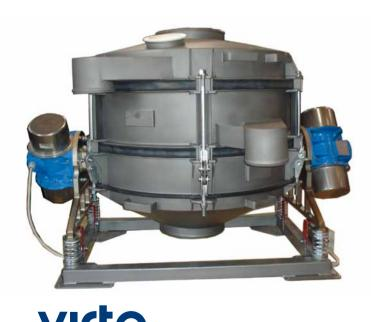
The ScreenX CD circular sieves are equipped with a double mesh cleaning device in multi-frequency vibration mode "MFVexcite". Especially effective for the separation of powders, granules and liquids considered non-screenable, obtaining the maximum screening efficiency and with the possibility of using mesh up to 20 microns.
