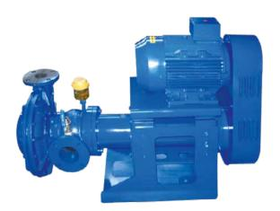
The horizontal centrifugal pumps, model EGO are manufactured especially for transferring highly abrasive fluids such as slurry, glaze, water with suspended solids etc. The oil bath seal or the water fluxing ensure lasting wear. The pump casing and the impeller are lined with special synthetic wear-resistant materials. The use of open impellers enables the transfer of large bodies without clogging.
