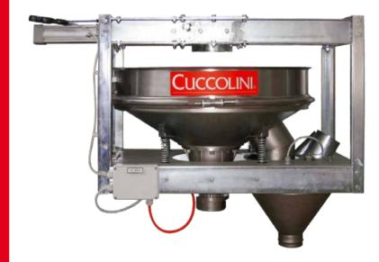
Atomised powder sieving unit behind the press. It is installed to feed the press car, consequently completely eliminating the risk of the formation of atomised lumps.
