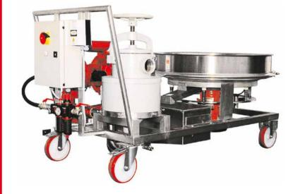
Wheel-mounted mobile unit for screening, transferring and removing iron from glaze.
