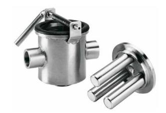
Iron-removing filter for fluids, operating under pressure and with permanent magnets. The compact size, the remarkable magnetic force of the Neodymium bars and the hermetic seal make the PZT 93-253 filter perfect for use on glazing lines, on service tanks and along glaze transfer piping.
