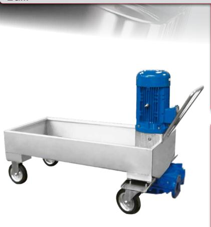
The tank is completely made o AISI 304 stainless steel and equipped with 4 support feet. The tank inner part has an inclined bottom to allow the product transfer on the pump aspiration side, keeping the tank bottom clean. The filtration grid installed inside the tank is made of AISI 304 stainless steel. The transmission is direct, the panel of the oversize shaft is made of anti-wear chrome.
